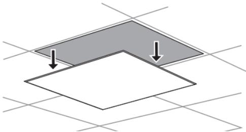
2. Place the Junction Box in the space above the suspended ceiling where you want to place the microphone array.
