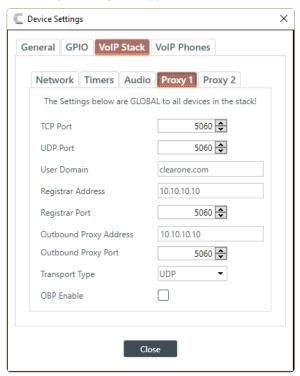
Type the domain and IP address of the proxy you are going to register to in the User Domain and Registrar Address fields. 10. Click the Audio tab.
